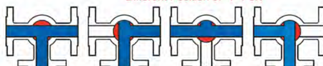
Different Position of "T" Port
