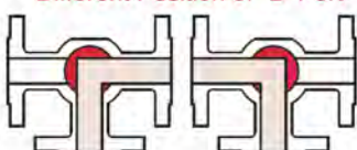
Different Position of "L" Port
